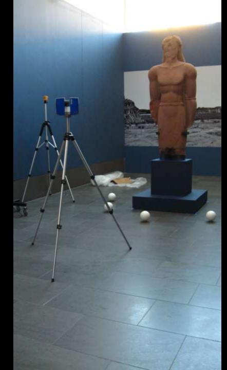
Testing for the sculptures inherent frequency or oscillating period.
